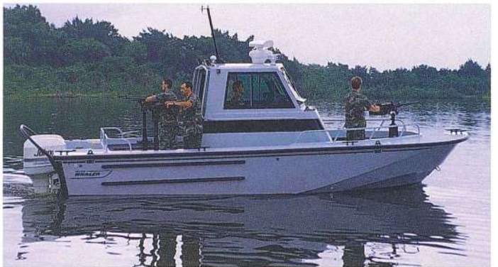
(Top: Note the convenient deck access of the Vigilant and the ample roof surface for mounting electronics. Middle: Shown with a tow post and twin 175's, this boat reaches speeds in excess of 30 knots with a 160 mile range with the standard 173 gallon fuel tank. Bottom: Optional gun mounts.)
