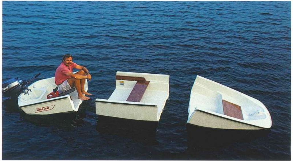
To demonstrate Boston Whaler's unsinkable Unibond™ construction, this 13 footer was cut into thirds.
