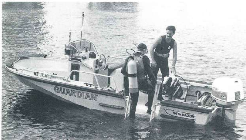
19' Guardian w/34" hull cutout, H.D. diver's ladder, rubbing strakes and console siren shelf. Note this boat has the older G II console system.
