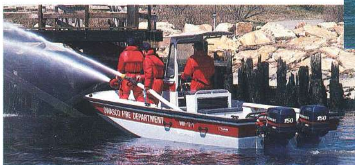
25' Guardian with 18 HP pump, weather protection "T" top and 34" rescue door.
