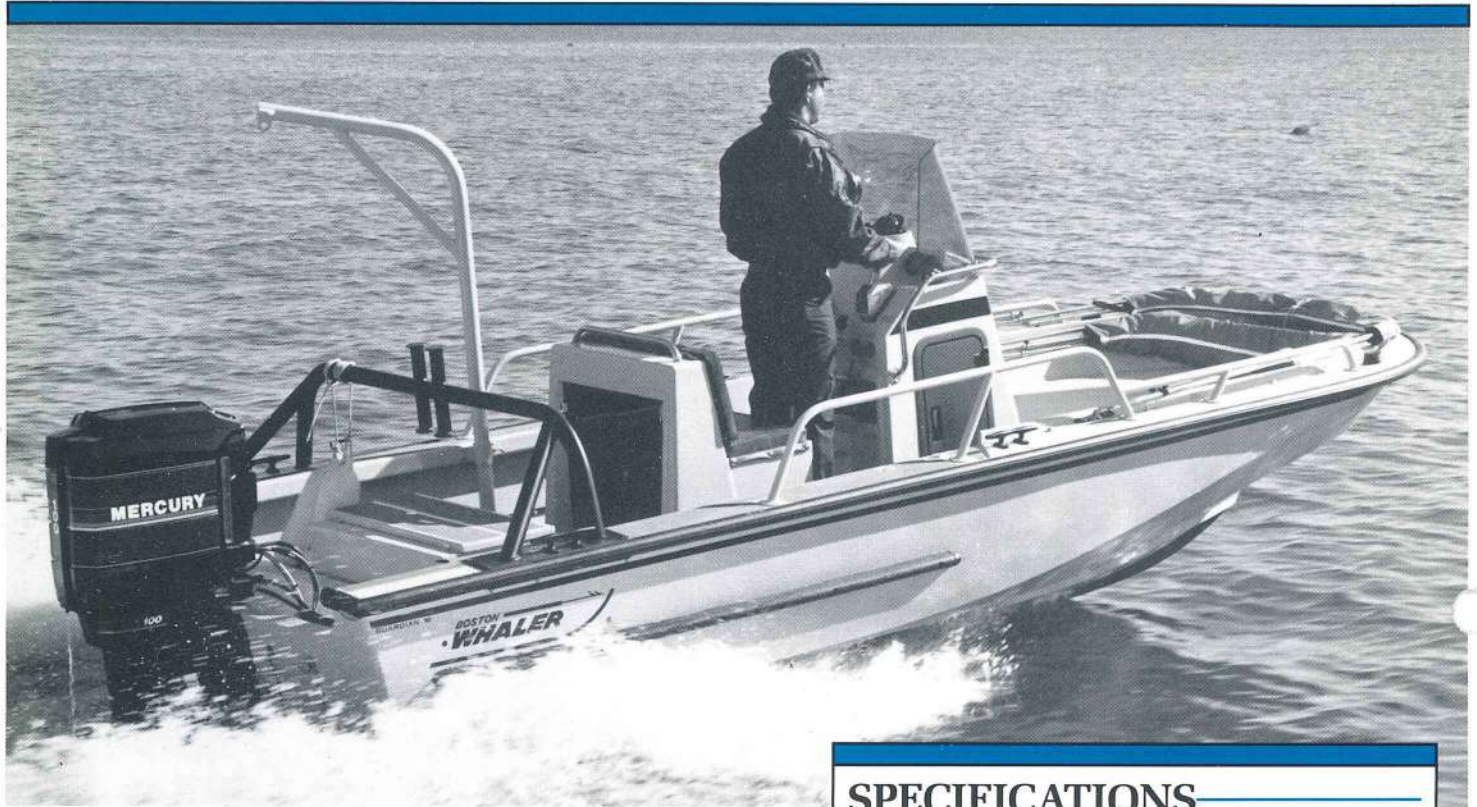
Guardian 19' with standard bench seat and optional davit and torsional tow bar. Canvas system is furled on the bow deck.
