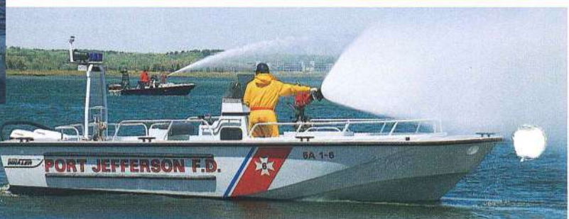
27' Guardian with 75HP fire pump, double rubbing strakes and custom graphics package.
