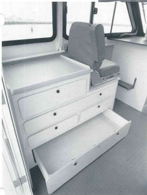
Custom cabinets provide storage for charts, manuals, and guns in the lower locker.
