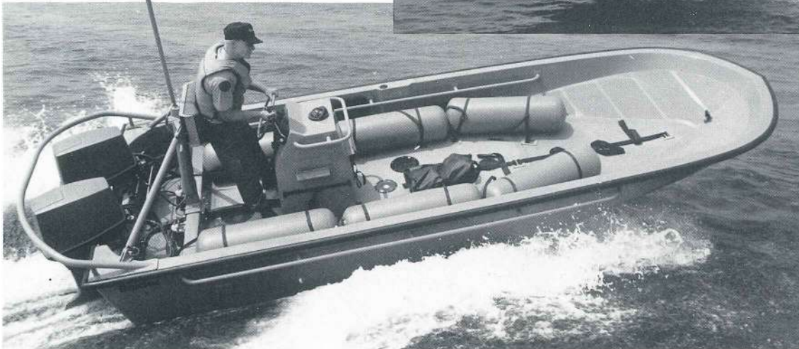
19' Rigid Raiding Craft with a carrying capacity of 10 troops, speeds well over 30 knots, and 54 gallons of fuel, this small assault craft can be launched from mother ships for over the horizon deployment. Keels, gunwales, and lifting hardware all have been beefed up for tough military service. Over 120 units are currently in service worldwide.
