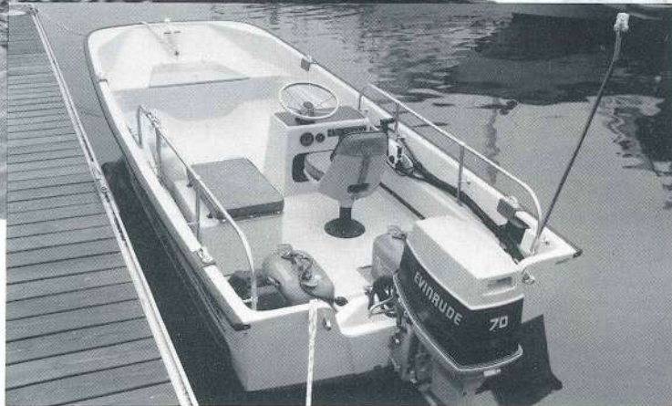
17' Utility w/70 H.P. outboard, swivel seat, and portside deck utility box.
