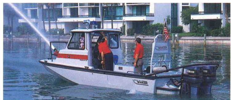
25' Frontier equipped with 75HP fire pump. Note: tow rail tower with crash screen protecting crew from recoil of failed tow-line or fitting.
