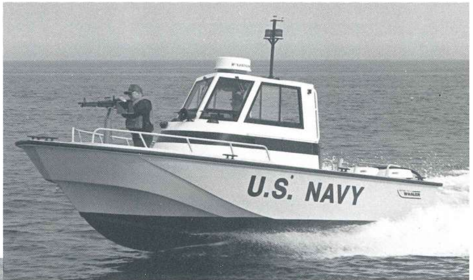
This shows the excellent field of fire available when the "plug in mount" is installed forward on the Vigilant 27'. Other security equipment includes a radar, strobe lights, and communications, all factory installed.
