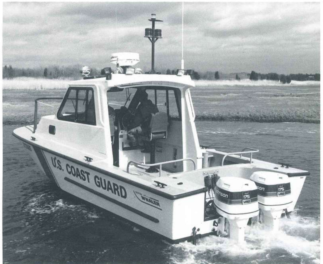
The standard rear drop curtain was completely removed in this photo to give a clear view of the helm station. Note the high pedestal seats which are standard. Options shown include, dual spotlights, radar, flood lights, strobe lights, Coast Guard graphics package and tow post.
