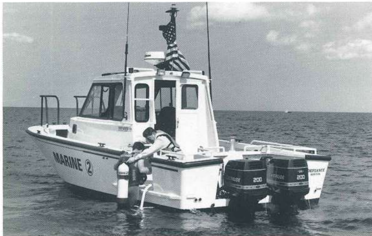
Dive door and ladder enhance the 30's rescue and recovery capabilities.
