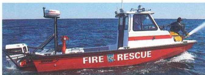
25' Frontier fireboat with full electronics and emergency lighting for night and low visibility fire/rescue operations.
