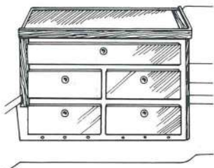
27' Challenger galley unit mounts on port side and features a large chart drawer and four storage drawers, top surface for chart work, etc.
