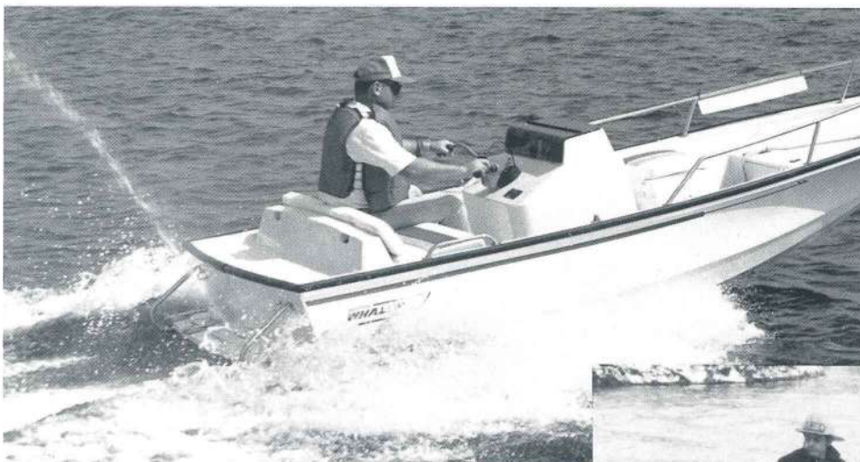
14' Jetboat equipped with center mounted console, forward anchor locker, low profile bow and side rails, and H.D. rub rail. Power is 50 H.P. Yamaha.
