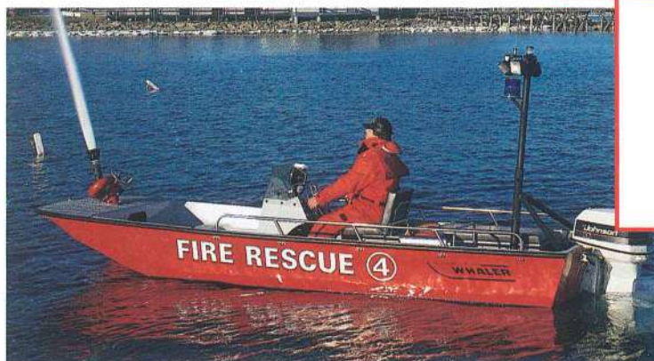
17' Utility with 18HP pump and starboard side console
