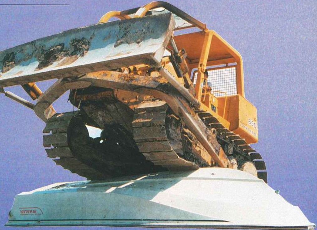
This 44,000 pound bulldozer is perched on top of a 19 foot Boston Whaler hull to demonstrate the strength of the Unibond™ construction process.
