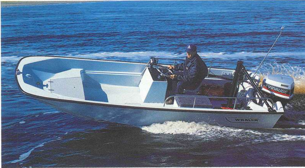
The Utility is well suited for shallow water operation or harbor patrol. Options on this 17' Utility include a swivel helm seat, deck utility box and a tow post.
