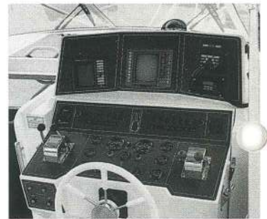
The steering console hinges for quick access while the three wraparound electronics panels give you plenty of space for all your instruments.
