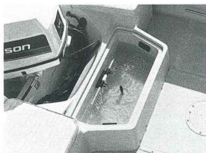
There's a covered storage bin forward of the engine that's convertible to a live well with an optional raw-water circulating kit.
