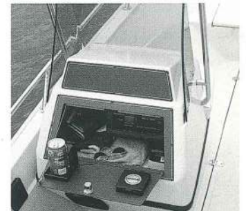
The port console has a fold-out table with drink holders and even more space for mounting electronics.
