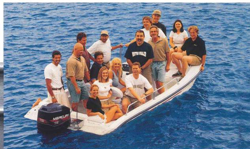
SWAMPED CAPACITY DEMONSTRATION. This 16' Boston Whaler was pumped full of water and it still kept 15 people high and dry. This illustrates Boston Whaler's extraordinary swamped capacity. Swamped capacity is defined as the amount of total weight a boat will support when filled with water.
