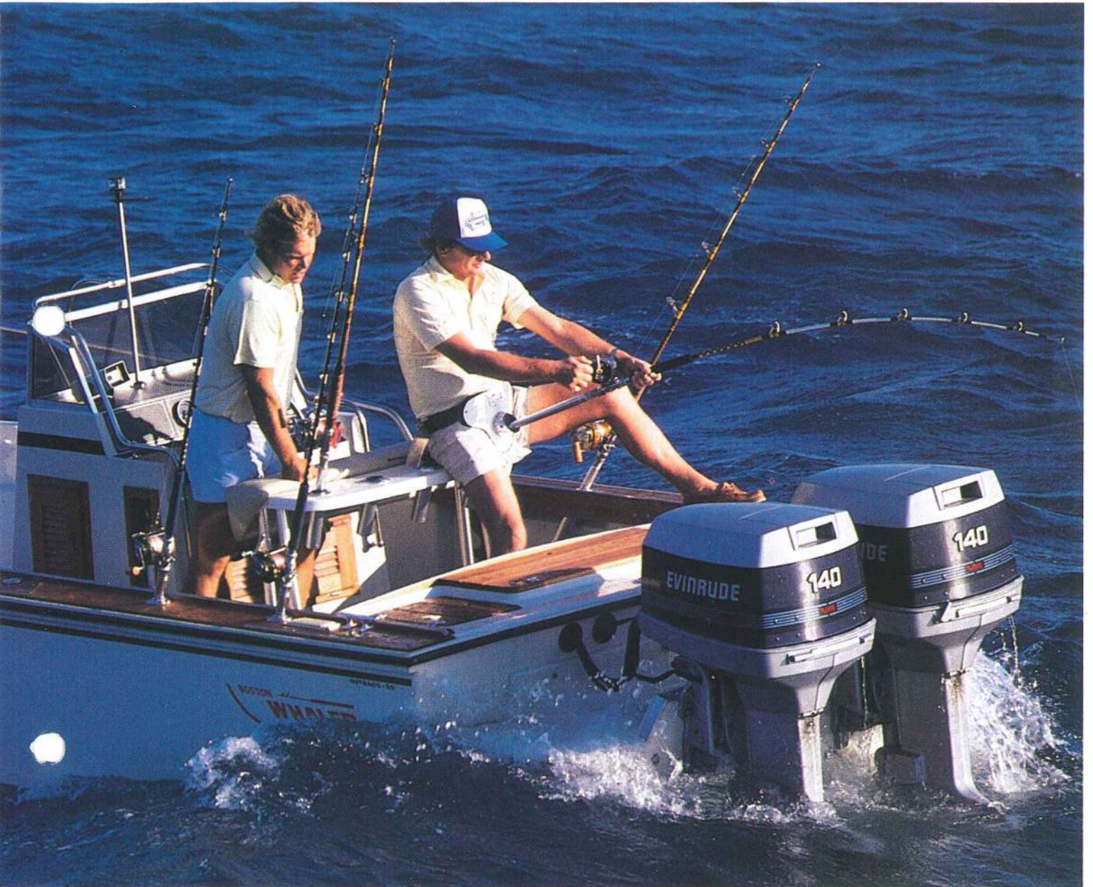
The Whaler Drive on this Outrage 20 allows more room in the cockpit, and adds two feet of extra length to the boat for a smoother ride.
