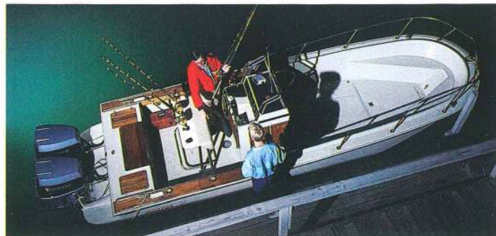
The Whaler Drive on this Outrage 20 allows more room in the cockpit, and adds two feet of extra length to the boat for a smoother ride.
