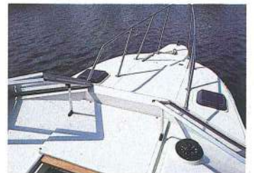
On Walk-Through models, an innovative bow rail that extends down the center of the boat from a walk-through windshield gives solid, sure-footed security for line handling, casting from the bow, or bringing aboard the anchor.
