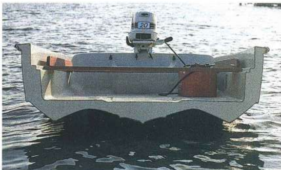
Unlike other boats with "foam flotation," ours is filled all the way to the gun'l's with a highly-compacted closed-cell foam. This means there are no voids where water can collect.
