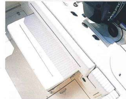
BOTTOM: Stern seat folds flush to transom for maximum cockpit space.
