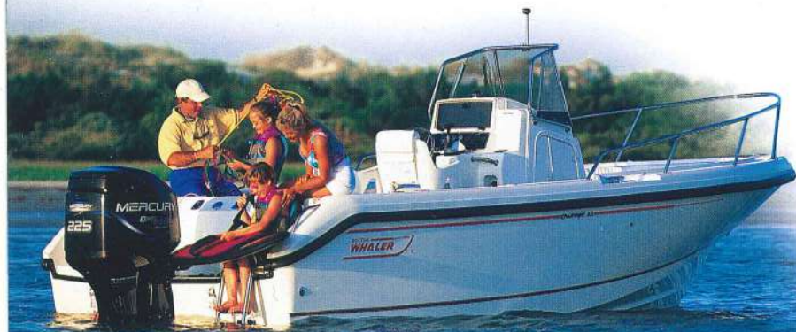
BOTTOM: Stern seat folds flush to transom for maximum cockpit space.
