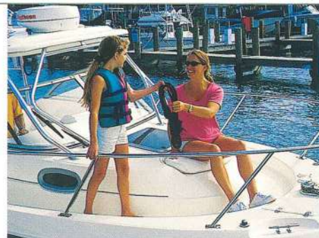
Whaler's traditionally straight sheerline is raised at the bow to accommodate a recessed walkaround without compromising cabin space. Here, a sturdy welded stainless steel bow rail aids in secure access to the anchor and bow seating area.
