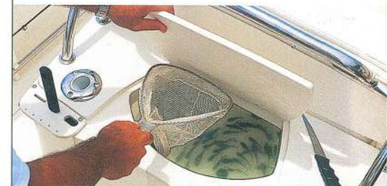
Under the cutting board of the optional deluxe leaning post is a recirculating livewell.
