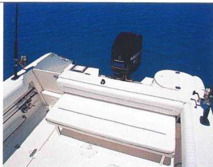
The stern seat folds into the transom to free up cockpit space.
