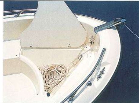
The bow contains a concealed storage / anchor locker with drain and a handy (optional) anchor roller.
