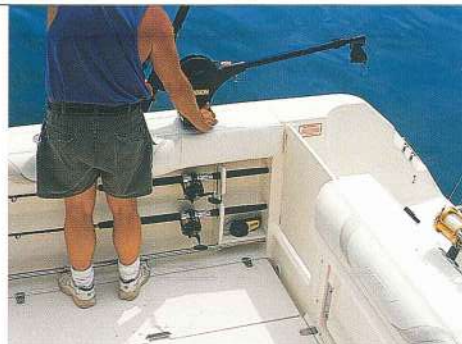
The 255 Conquest is built to fish, with a hideaway stern bench seat that folds into the transom to free up space, under-gunnel rod racks above stainless steel toe rails, port and starboard downrigger weight holders, and much more.
