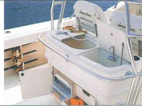
Prep station includes two sinks, fresh and raw water, cutting board and tackle drawers.
