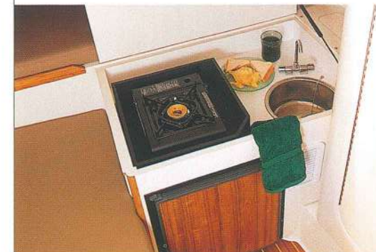
Optional Galley Package features a butane or electric burner, sink with hot and cold pressure water and refrigerator.
