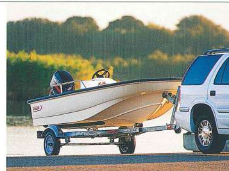
The standard galvanized trailer features a winch with nylon strap, tie-downs and a trailer jack.
