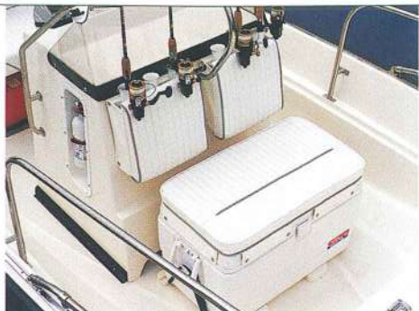
Convenient rod holders with cushions serve as backrests for the cooler seat.
