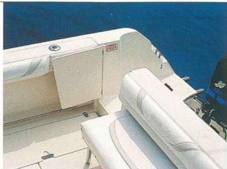
The stern area provides a walk-thru transom door with stainless steel latch for quick and easy access to the boarding platform and telescoping stainless steel swim ladder.
