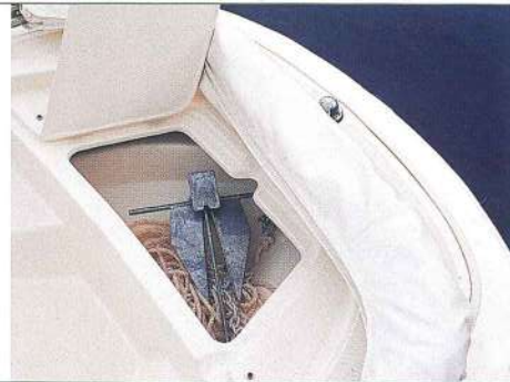
The bow locker with fiberglass cover and drain keeps the anchor and gear out of the way.
