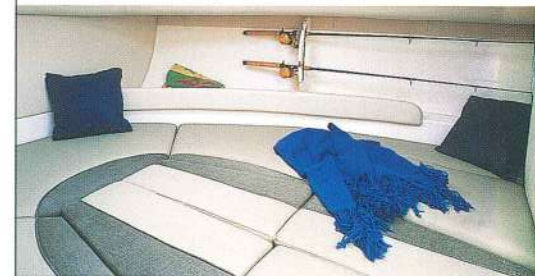
The optional table doubles as a filler that converts the V-berth settee into a double berth.
