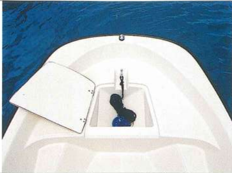
The bow locker with fiberglass cover and drain keeps the anchor and gear concealed.
