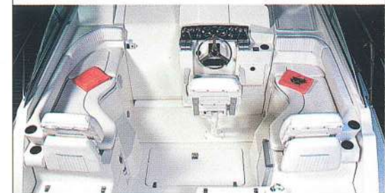
Cockpit has complete instrumentation, custom switch panel, dual-lever engine controls and port and starboard L-shaped lounge seating.
