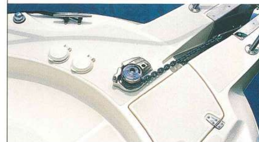
The oversized anchor locker provides plenty of space for anchor and rode. The low-profile windlass with rode is available as an option.
