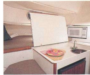
28' OUTRAGE: Galley package includes single burner stove (butane or electric) refrigerator (12V/110V) and stainless steel sink with hot / cold pressurized water.
