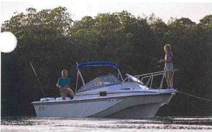
The Revenge 25's walk-through windshield and extended bow pulpit afford easy access to the bow.
