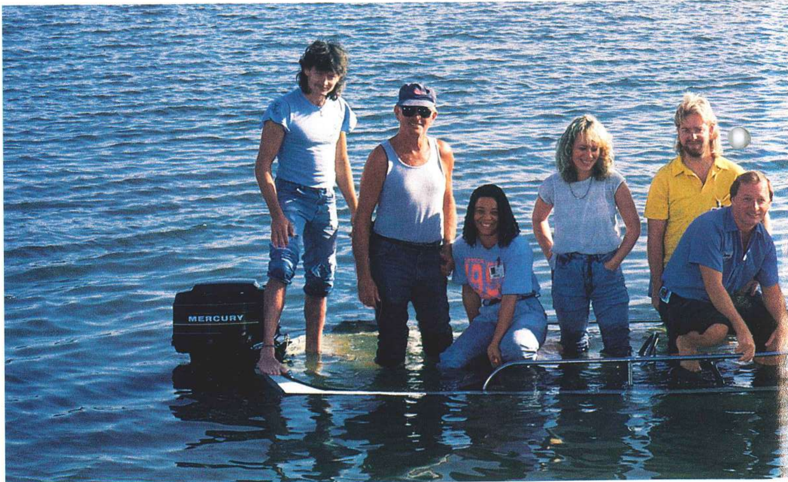
You can pack up to 1,600 pounds into a 13' Boston Whaler; then pull the plug, and it'll float high enough to keep the engine dry.
