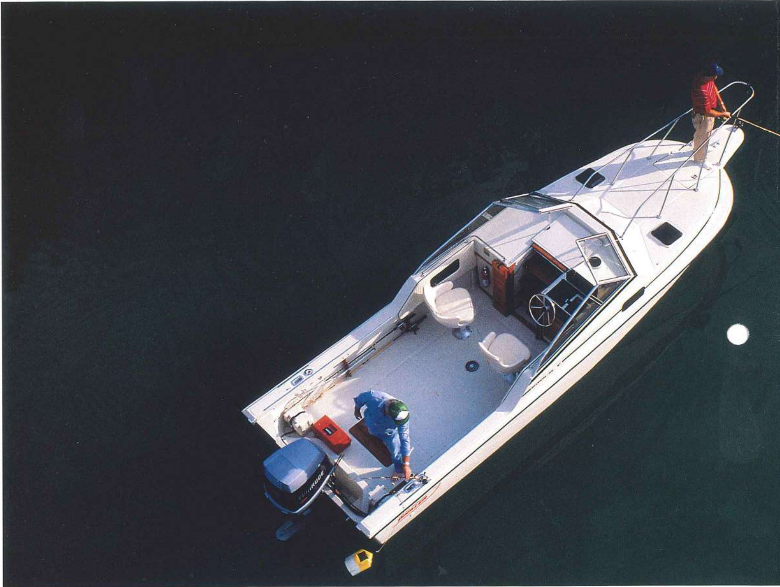
The Revenge 22 has a deep-Vee hull, for a smooth, comfortable ride.
