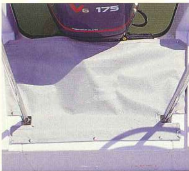
The mesh motorwell net prevents snagging lines on rigging.
