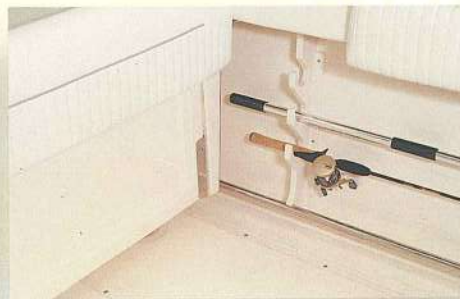
The stern seat folds flat against the transom for additional cockpit space.
