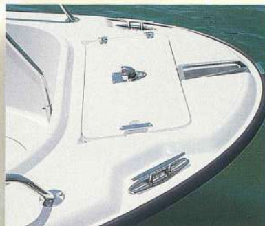
Standard navigation lights, pull up cleats and anchor locker.
