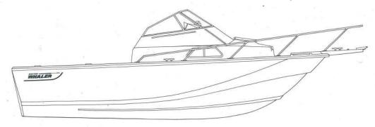
Key Specifications: LOA 25'3" (27'11" with Whaler Drive<sup>™</sup>). Beam 9'6". Draft 18". Boat weight 5,500 lbs. Max. weight capacity (persons, motor and gear) 4200 lbs. Swamped capacity 10,000 lbs. Persons capacity 12. Max. horsepower 550. Transom height 25". Sleeps 3. Fuel 250 gal.
