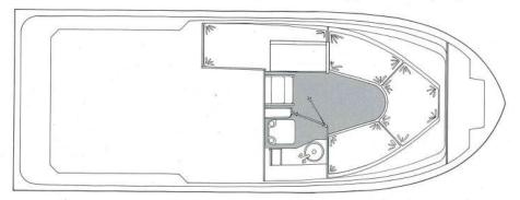
Partial list of cabin standard features: Cabin: Lighted V-berth and quarter berth. Under bunk storage. Dinette. Cushions. Fold-down galley counter. Rod storage. Head: Fully enclosed and lighted. Sink w/pressure system. 15-gallon water tank. Head w/deck pump out/overboard. Vanity w/overhead cabinet.
