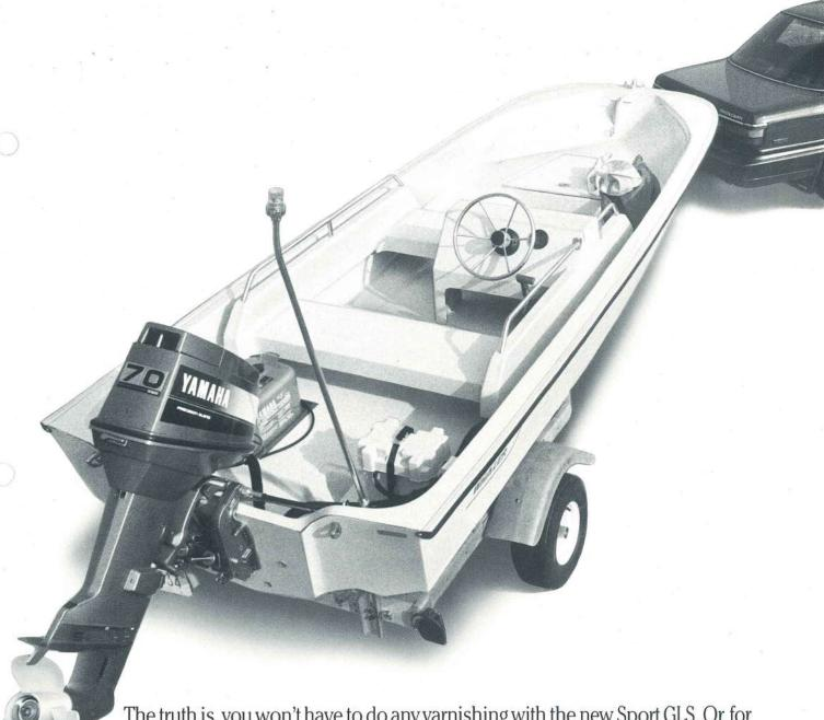
The truth is, you won't have to do any varnishing with the new Sport GLS. Or, for that matter, any sanding, scraping or stripping. For we've added a low-maintenance fiberglass interior to our legendary Sport hull. The same unsinkable hull of closed-cell foam and fiberglass that boat owners have come to rely on for over three decades.
